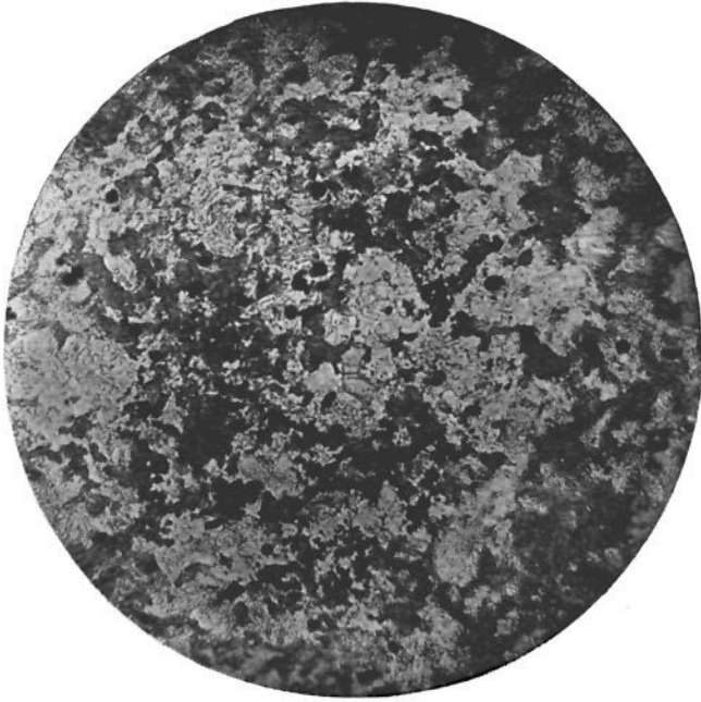
Fig. 1.—Dakota mustard flour, X 110. Dark spots show starch grains of foreign weed-seed, stained with iodine.
